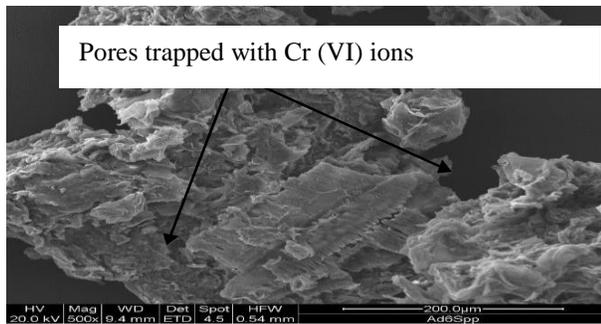
Figure 3b: SPP after adsorption.
