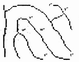
Fig. 7d. Thinning with a combination of Stentiford's smoothing procedure, Zhang-Suen's algorithm and Holt et al's staircase removal scheme.
