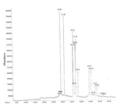
Figure 2: GC chromatogram of 1% KOH biodiesel.
