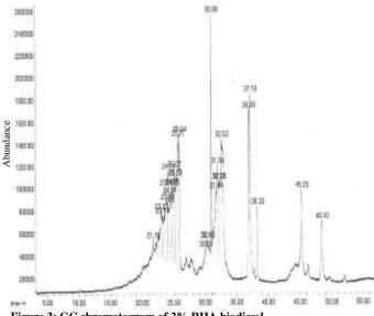
Figure 3: GC chromatogram of 2% RHA biodiesel.
