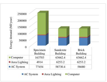
Figure 10. Cumulative exergy consumption of the specimen building and the variants of control building.
