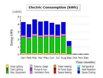
Figure 8. Monthly Electrical consumption by End use in the Burnt Brick Building
