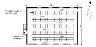
Figure 2. The typical layout plan for the specimen building and control building.
