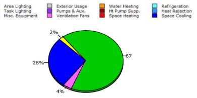
Figure 5. The Annual Electric Consumption by End-use of the Specimen Building.
