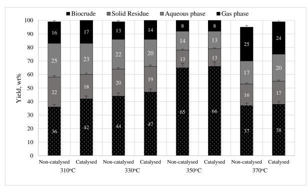
Figure 1: Products derived from HTL of microalgae with and without catalyst at different reaction temperature.
