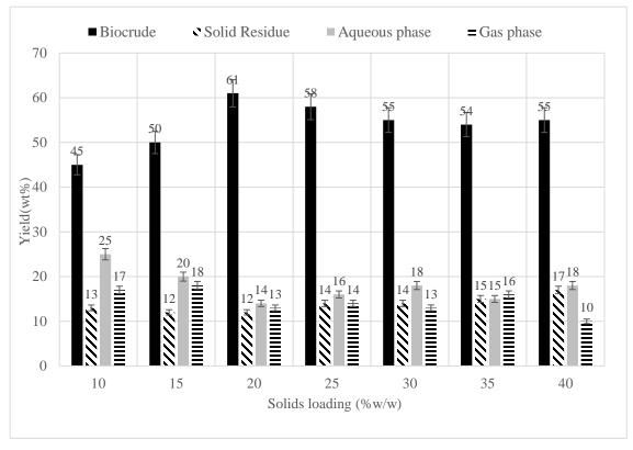
Figure 2: Phase yields obtained from HTL of halophytic Tetraselmis sp. microalga at different solids loading at 350°C.
