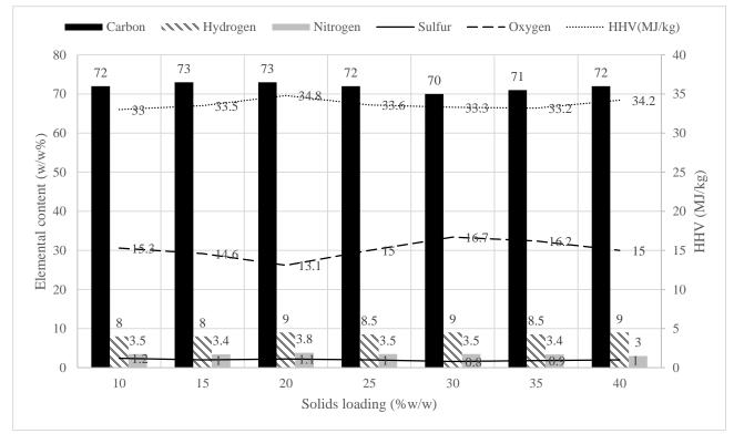
Figure 3: Elemental content and energy density of biocrude after HTL of halophytic *Tetraselmis* sp. microalga at different solids loading at 350°C.
