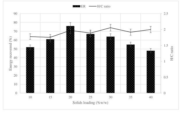
Figure 4: Energy recovered and H/C ratio in biocrude obtained at different solids loading.
