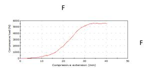
Figure 1f: Influence of Tillage Practice F on Compression Test of TMS 0581 Cassava Tubers for a Rain Fed Soil + 622.50 kg/ha Fertilizer.
