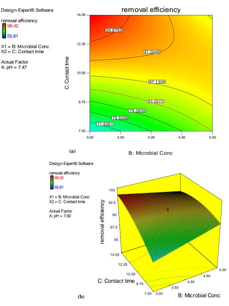
Figure 5: 3-D surface and contour plots of  $E_R$  with contact time and Microbial concentration. (a) contour map (b) surface plot.
