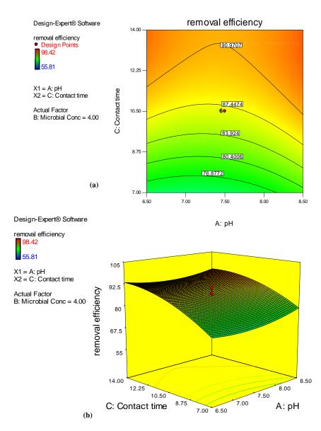
Figure 7: 3-D surface and contour plots of  $E_R$  with contact time and pH (a) contour map (b) surface plot.
