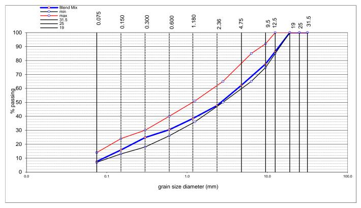
Figure 1: Aggregate grading curve.
