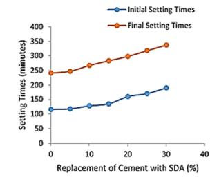
Figure 4: Initial and final setting times of paste with SDA (Elinwa & Ejeh, 2004.).
