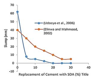
Figure 5: The slump characteristics of concrete with SDA.
