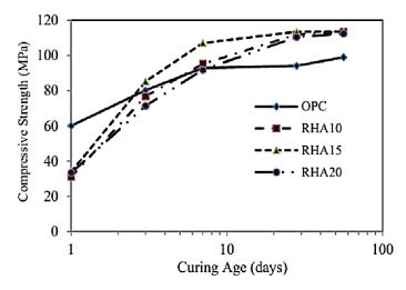
Figure 2: Effect of RHA on the compressive strength of concrete (Mahmud *et al.*, 2016).
