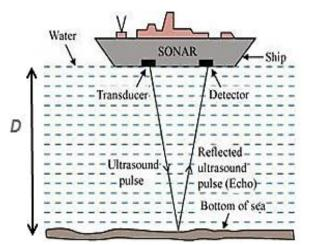
Figure 3: Principle of acoustic depth measurement: Sources: (Arseni et al., 2016).
