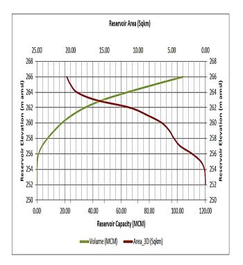
Figure 4: Lugu dam reservoir area-elevation-capacity curve.
