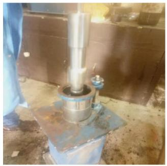
Figure 3: Sample of Asphalt concrete in the compaction mould.
