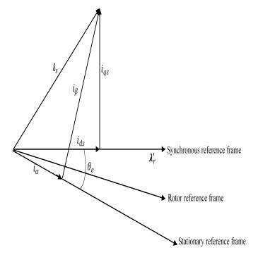
Figure 1: Rotor flux vector alignment with the d-axis.
