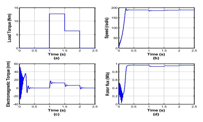
Figure 4: Simulation results of the motor behavior (a) Load torque with Time (b) Speed with Time (c) Electromagnetic torque with Time (d) Rotor flux with Time.
