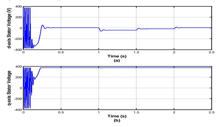
Figure 7: Direct and quadrature axis voltages in the stator.
