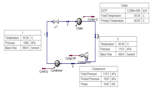
Figure 7: Propane refrigeration loop sub-flowsheet.
