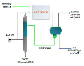
Figure 2: IFPEX-1 Flow Scheme.
