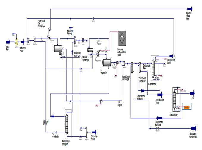
Figure 6: Process Flow Diagram of the IFPEX-1 process and NGL fractionation columns in ASPEN HYSYS V9.
