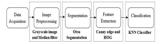
Figure 1: Block diagram of the developed system.
