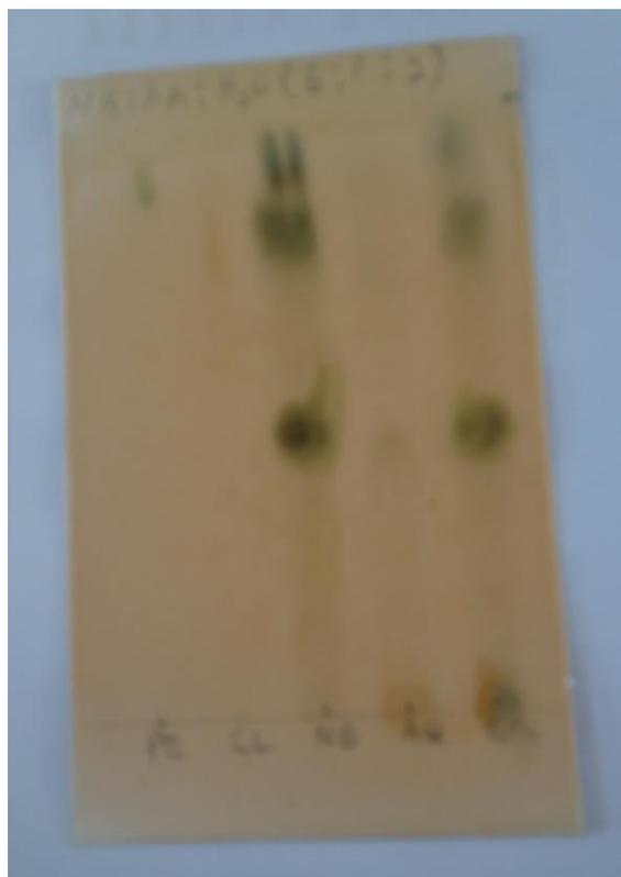
**Plate 1: TLC plate after spraying the various fractions eluted in the solvent system (6:1:2) with Ferric chloride. Note the greenish spots indicating the presence of phenols and flavonoids.**
