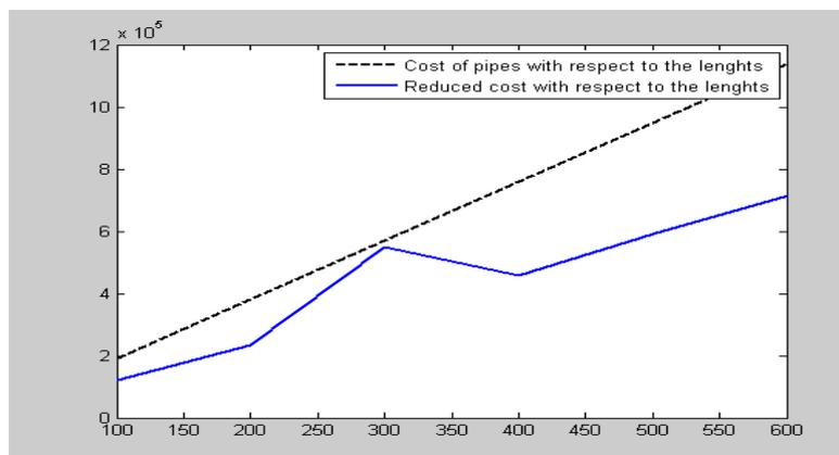
**Figure 1:** Actual cost and reduced cost for a pipe diameter of 2.56 inches and various lengths
