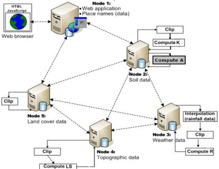
Figure 5: Processing steps for calculating the annual average of the soil loss
