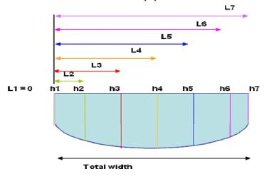
*Figure 2: Diagramme of cross section survey (Author, 2009)* Where: Li: cross sectional width, hi: heigh
