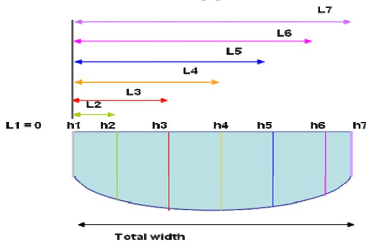
Figure 2: Diagramme of cross section survey (Author, 2009)
