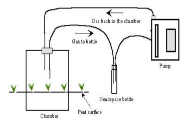
Figure 1 Experimental set up to collect the GHG sample from the field
