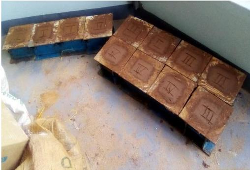
Figure 4: Cubes in the moulds
