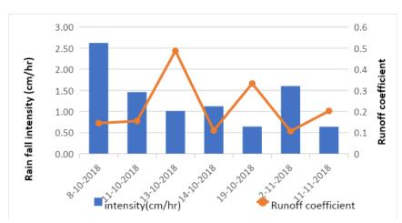
Figure 12. Rainfall fluctuations and variability of runoff coefficients for MF Plot
