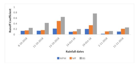
Figure 6. Effect of land cover on runoff coefficient
