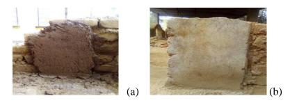
Figure 9: Plastered cohesive soil mortar mixed with the cow dung (a), and plastered cement mortar
