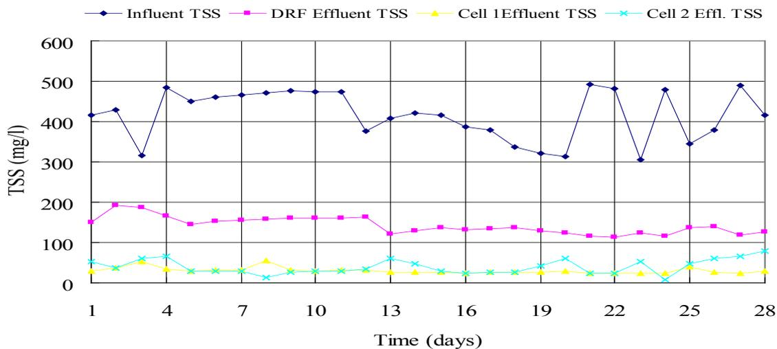
Figure 4. Daily variation of inflow and outflow TSS in DRF and HSSFCW cells
