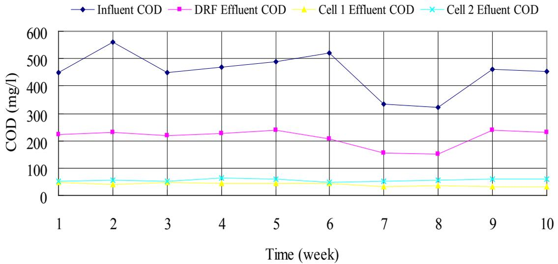
Figure 5. Weekly variation of chemical oxygen demand in HSSFCW cells
