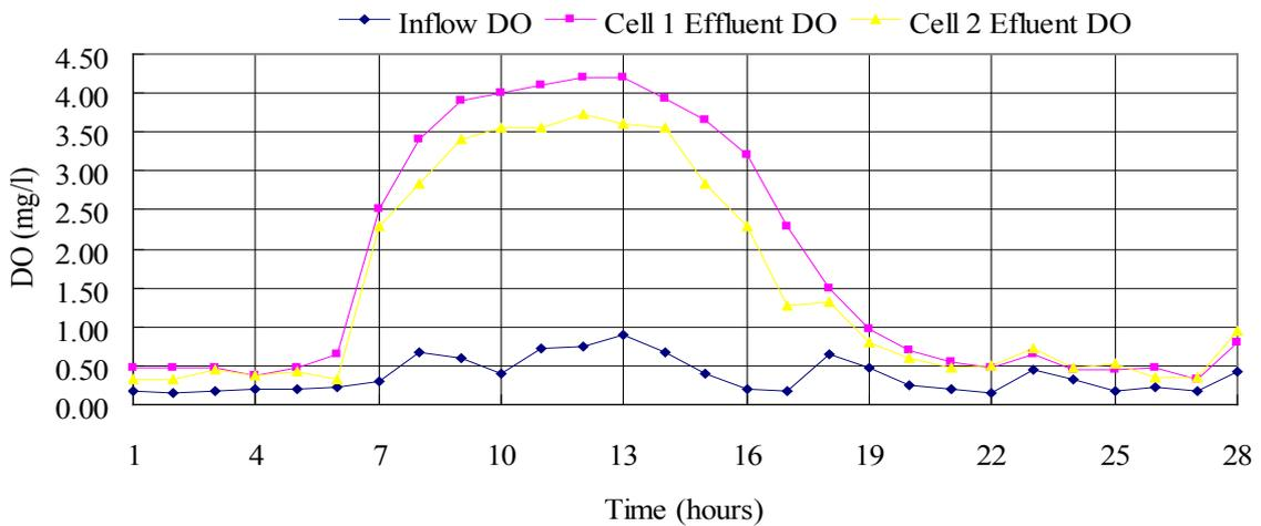
Figure 7. Hourly variation of DO in the HSSFCW cells
