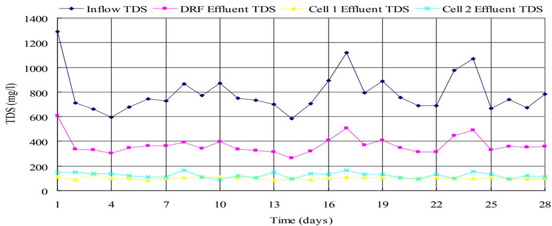
Figure 3. Daily Variation of total dissolved solids in DRF and HSSFCW cells
