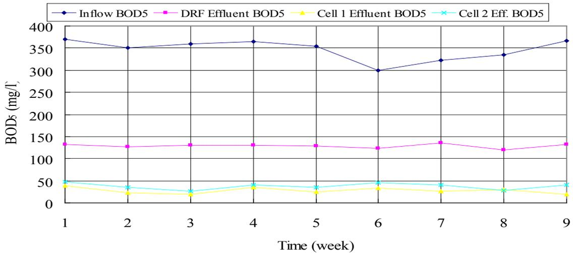
Figure 6. Weekly variation of BODs in HSSFCW cells
