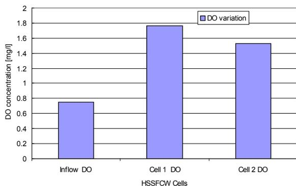
**Figure 8: Average Dissolved Oxygen (DO) effluents from HSSFCW cells 1 and 2 planted with macrophytes**
