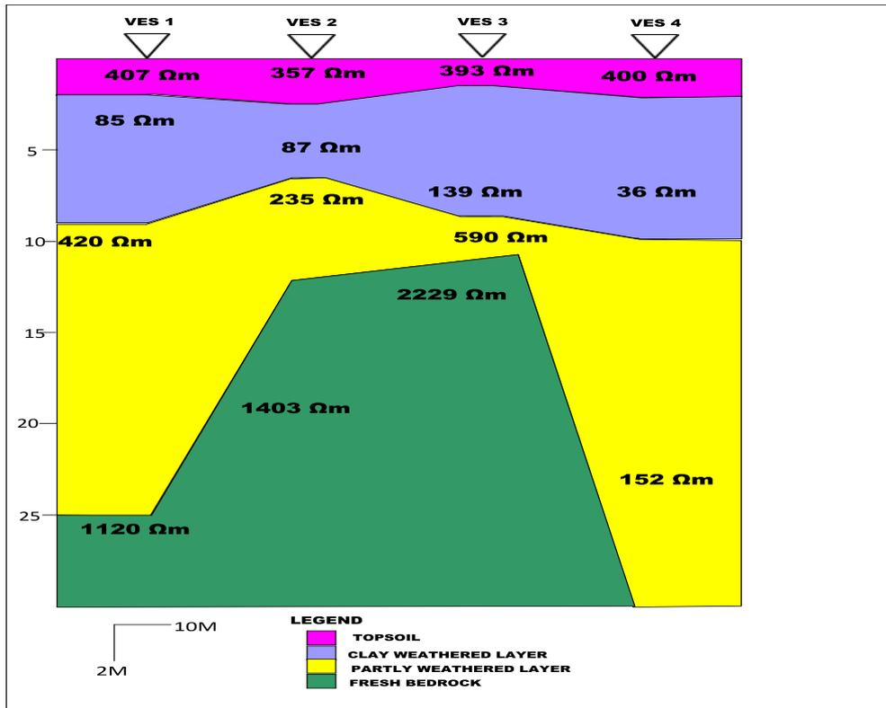
**Figure 4:** Goelectric section of Profile one
