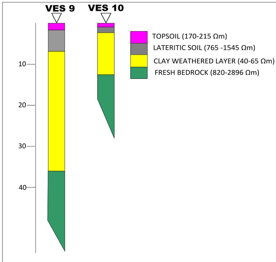
**Figure 6:** Geoelectric section of VES 9 and 10
