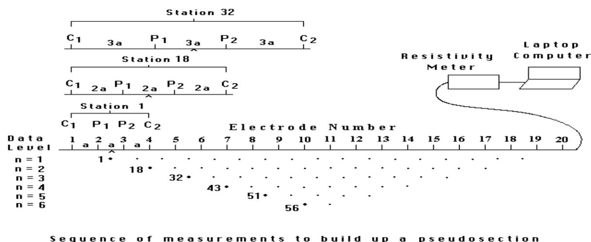
**Figure 3:** Illustration of 2-D electrical imaging set-up
