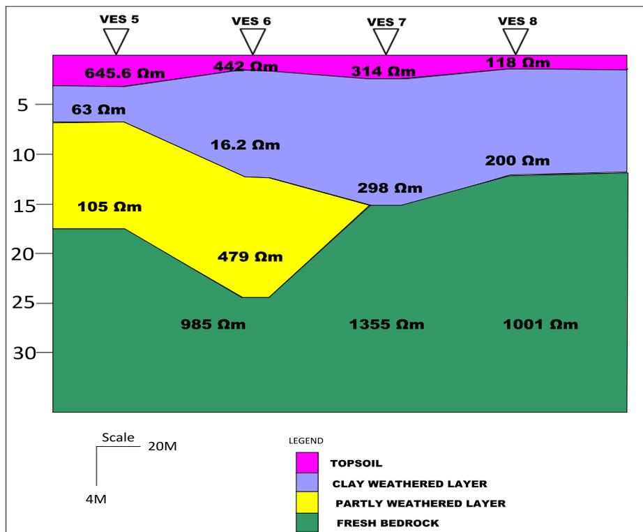
**Figure 5:** Goelectric section of Profile two.
