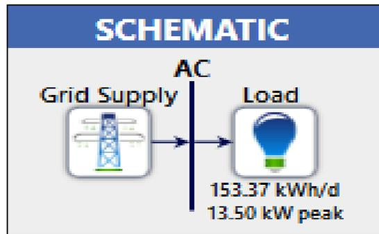
Fig. 2. Grid supply and load model in HOMER
