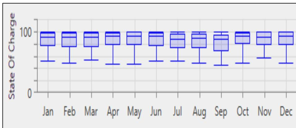
Fig. 9. SOC for the grid, PV and generator system
