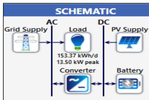
Fig. 4. Grid and PV supply model in HOMER
