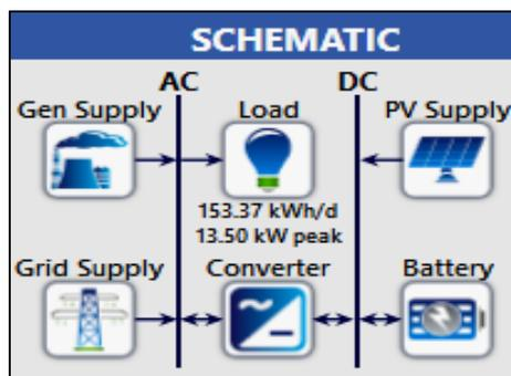
Fig. 7. Grid, PV and generator system supply model in HOMER
