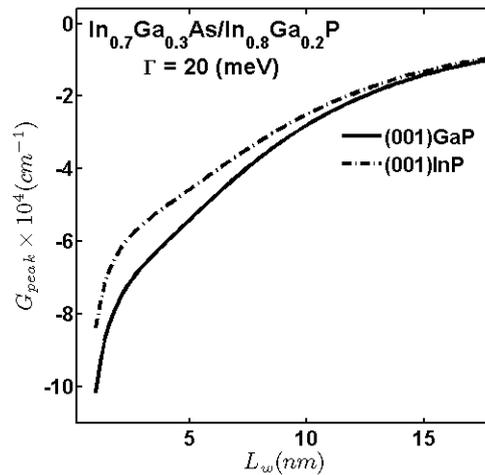
Fig. 7: Peak gain  $\alpha_{peak}$  against quantum well width  $L_w$  (nm).
