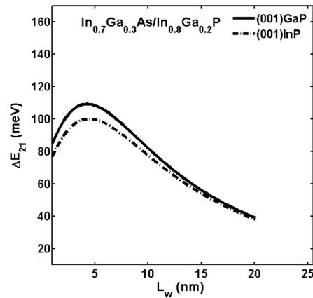
Fig. 4: Transition energy of  $E_{21}$ (meV) against quantum well width  $L_w$ (nm).
