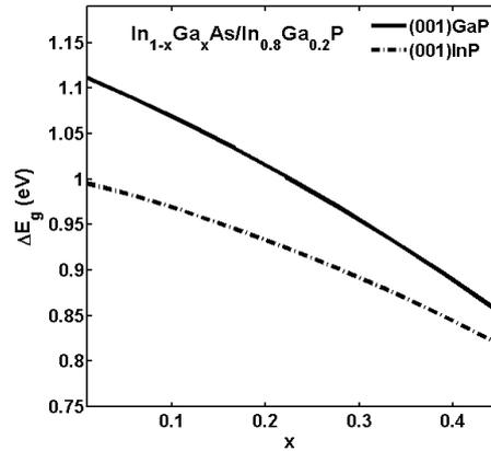
Fig. 2: Change in heavy hole bandgap  $\Delta E_g$ (eV) against Ga mole fraction  $x$ .
