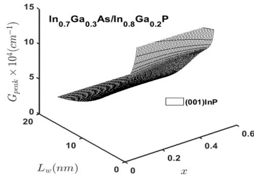
Fig.9: 3D mesh of the  $\alpha_{peak}$  against Ga mole fraction,  $x$  and quantum well width  $L_w$  for (001) InP substrates.
