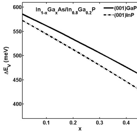
Fig. 1: (a) Heavy hole valence band offset  $\Delta E_v$ (eV) against Ga mole fraction  $x$ .
