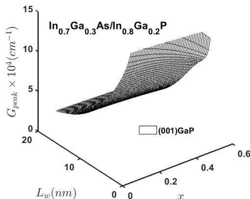
Fig. 8: 3D mesh of the  $\alpha_{peak}$  against Ga mole fraction,  $x$  and quantum well width  $L_w$  for (001) GaP.
