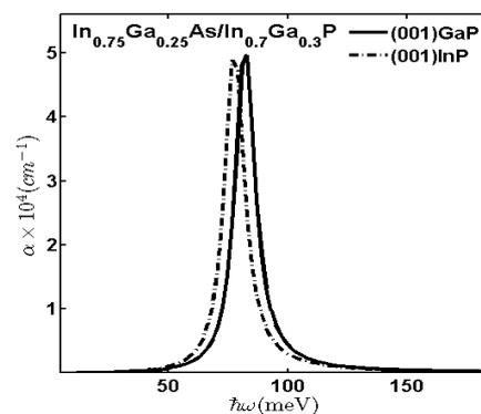
Fig. 6: Optical absorption spectra  $\alpha(\omega)$  against photon energy  $\hbar\omega$ .
