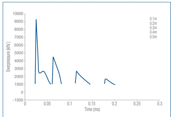
Figure 5: Simulated overpressure predictions at various distances from the grenade
