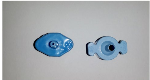
Figure 1: Defective connector with narrowed lumen (right) compared with a normal connector of size 3.5 mm ET (left).
