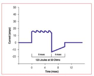
Figure 7: A typical rectilinear biphasic waveform
