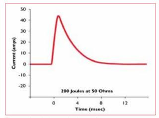
Figure 5: A typical monophasic waveform
