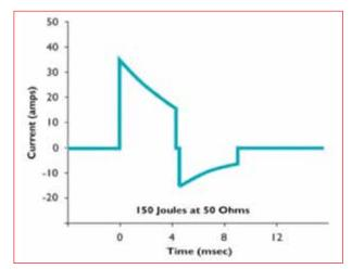
Figure 6: A typical BTE waveform
