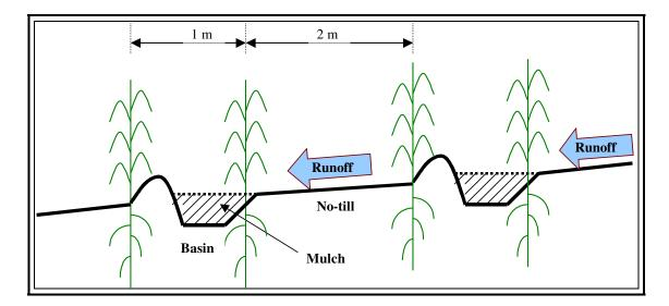
Figure 1: Diagrammatic representation of the Infield Rain Water Harvesting (IRWH) technique (after Hensley, *et al*, 2000)
