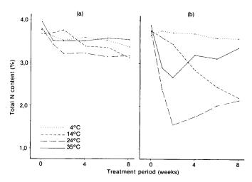
Figure 1 The total N content of urea ammoniated wheat straw after various treatment periods at four temperatures and at moisture levels of 250 g/kg wheat straw (a) and 375 g/kg wheat straw (b).
