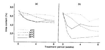
Figure 2 The urea content of urea ammoniated wheat straw after various treatment periods at four temperatures and at moisture levels of 250 g/kg wheat straw (a) and 375 g/kg wheat straw (b).
