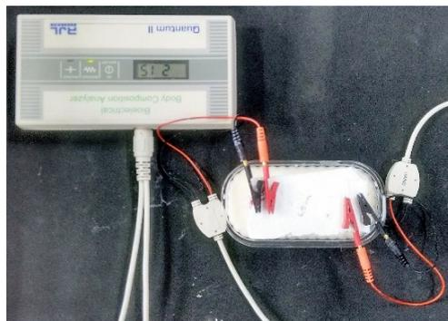
**Figure 1:** Representative methodology of electrical bioimpedance measurements in bovine raw milk
