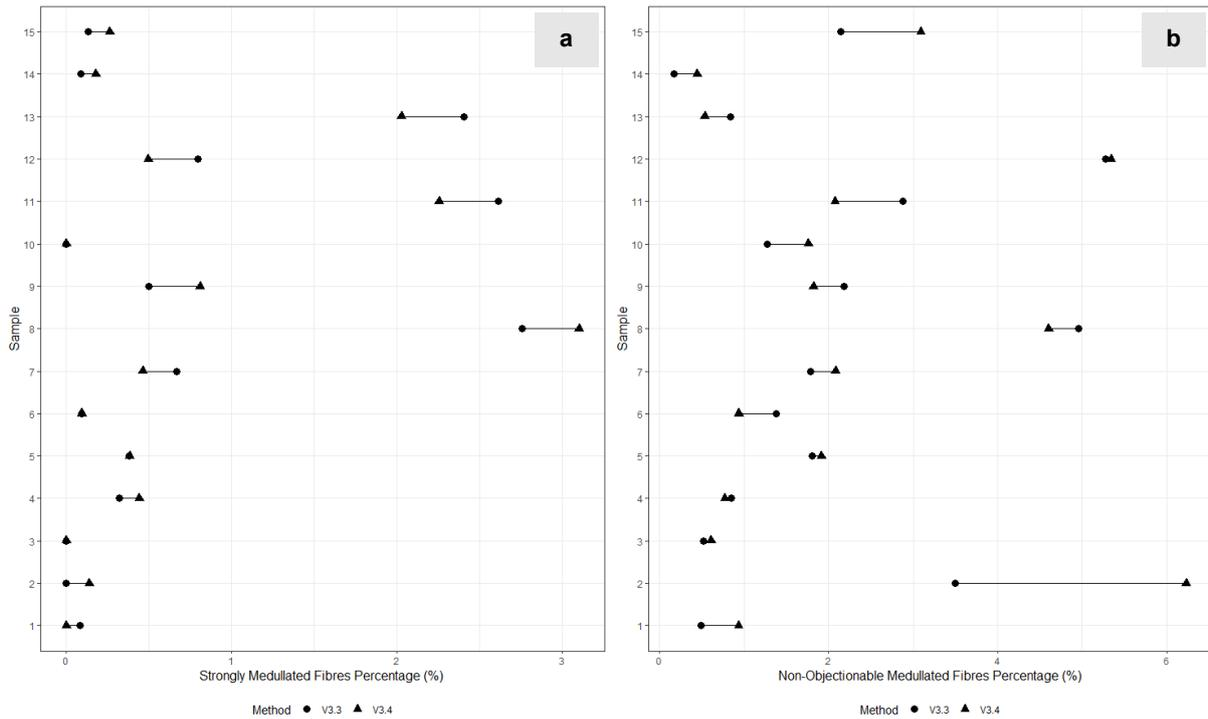
**Figure 3** Dumbbell plots comparing the counts performed by two different AI models of image analysis (v3.3 ● and v3.4 ▲) for (a) strongly medullated fibres and (b) non-objectionable medullated fibres in mohair samples.
