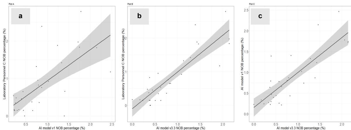
**Figure 6** Scatter plots of counts performed by laboratory personnel C and AI models of image analysis v1 and v3.3 for non-objectionable medullated (NOB) fibres in mohair samples (a: C versus v1, b: C versus v3.3, c: v1 versus v3.3).
