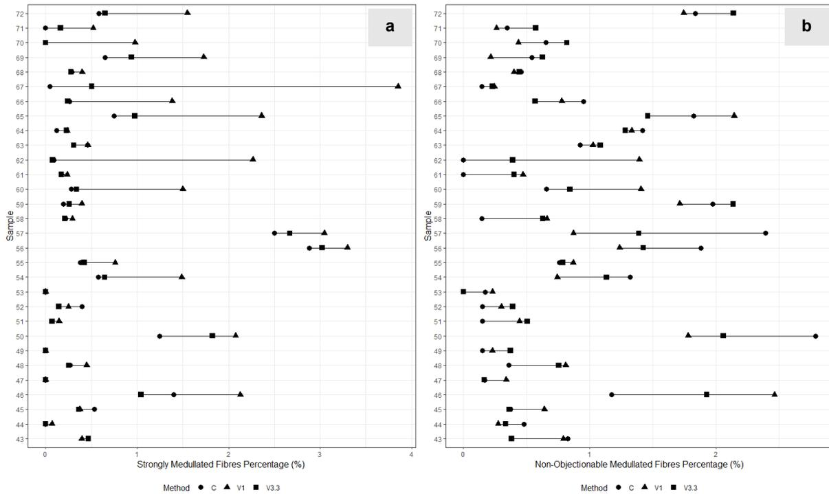
**Figure 2** Dumbbell plots comparing the counts performed by laboratory personnel C (●), and AI models of image analysis v1 (▲) and v3.3 (■), for (a) strongly medullated fibres and (b) non-objectionable medullated fibres in mohair samples.
