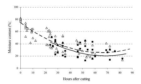
**Figure 2** The moisture content (x hours after cutting) of lucerne dried naturally ( $\Delta$ ) (Y = 39.51 - 0.789 (x - 30.65) + 0.0114(x - 30.65)<sup>2</sup>) and in the bulk drier (**■**) (Y = 36.76 - 0.870 (x - 30.65) + 0.0116(x - 30.65)<sup>2</sup>).
