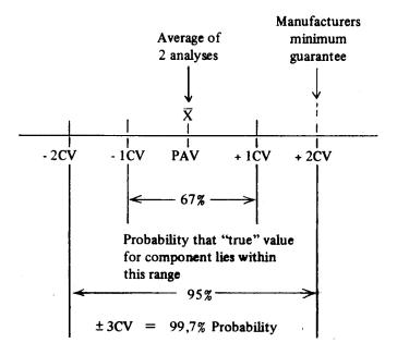
Fig. 1 Probability of "Truth" of analytical measurement (duplicate determination average) as compared to minimum guarantee for that component
