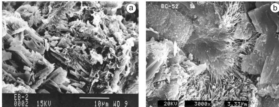
**Figure 2** SEM photomicrographs of zeolitic tuffs added to litter: a) Platy clinoptilolites surrounded with smectite flakes, b) Bundles of radiating mordenite needles developed in the matrix, and platy clinoptilolites and prismatic feldspars
