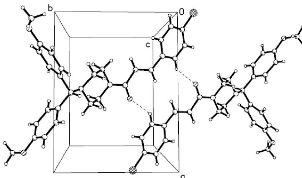
**Figure 2** Part of the crystal structure of (*E*)-1-{4-[bis(4-methoxyphenyl)methyl]-piperazin-1-yl}-3-(4-chlorophenyl)prop-2-en-1-one showing intermolecular hydrogen bonds.
