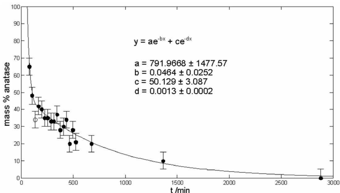
**Figure 2** A two-term exponential fit of the mass percentage anatase, determined from PXRD analysis, plotted against the reaction time.
