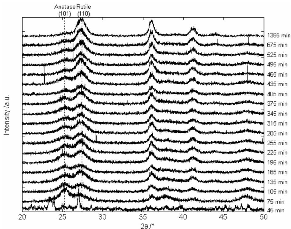
**Figure 1** PXRD patterns of the samples showing the formation of anatase from a complex precursor and the conversion of anatase to rutile. This conversion is observed through the changing ratios of the maximum intensity of the anatase (101) Bragg peak at  $25.4^\circ 2\theta$  and the rutile (110) peak at  $27.5^\circ 2\theta$ .
