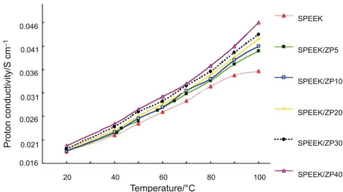
Figure 7 The proton conductivity of SPEEK/ZP membranes as a function of temperature.
