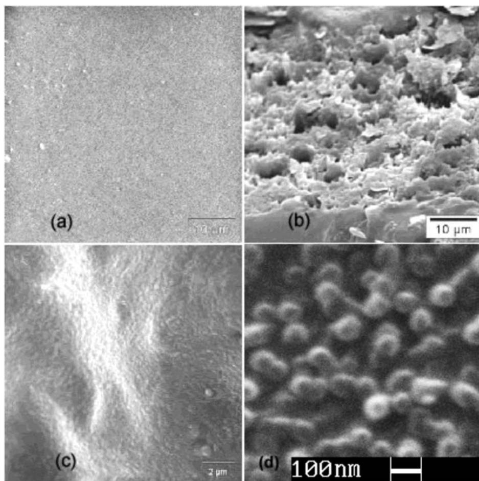
**Figure 6** SEM micrographs of SPEEK and SPEEK/ZP composite membrane: (a) surface of the SPEEK membrane, (b) cross-section of the SPEEK membrane, (c) surface of the composite membrane with 5 mass % of ZP, (d) cross-section of the composite membrane with 5 mass % of ZP.
