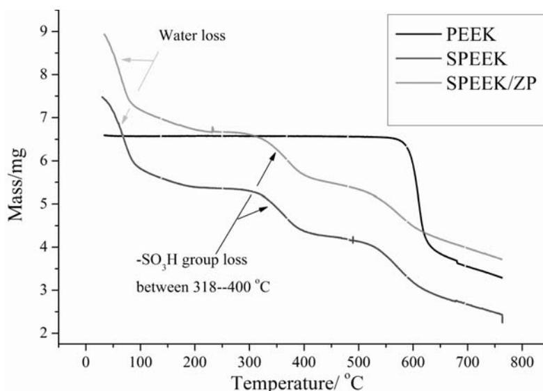
**Figure 3** Thermo-gravimetric curves of PEEK, SPEEK and SPEEK/ZP.
