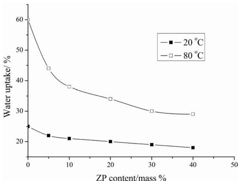
Figure 4 Water uptake of the membranes with different ZP content.
