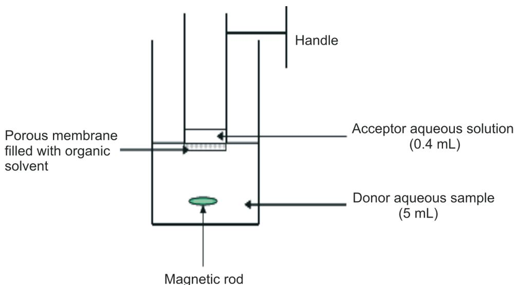
Figure 1 The set-up of the supported liquid membrane extraction probe.
