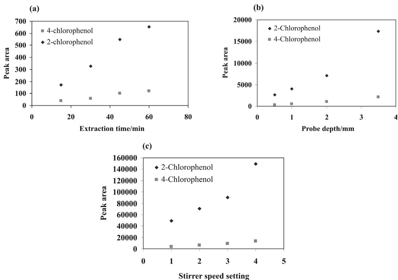
**Figure 3** (a) Optimization of the extraction time results; (b) optimization of the probe depth results; (c) optimization of the stirring speed results.
