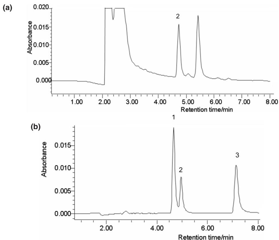
**Figure 5** Comparison of chromatograms of the extraction of chlorophenols (a) in a landfill leachate and (b) obtained from direct injection of  $0.1 \text{ mg L}^{-1}$  standard mixture. Absorbance measured at 280 nm.
