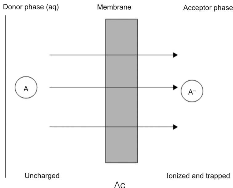
**Figure 2** Theory of the extraction process.  $\Delta C$  denotes the concentration gradient.
