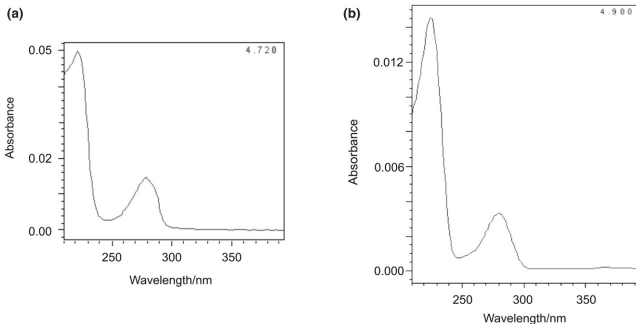
**Figure 4** Comparison of UV spectra of 4-chlorophenol obtained from (a) landfill leachate sample and (b) standard mixture.
