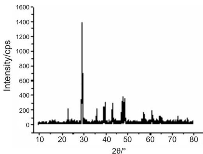
Figure 3 XRD spectrum of CaCO<sub>3</sub>.
