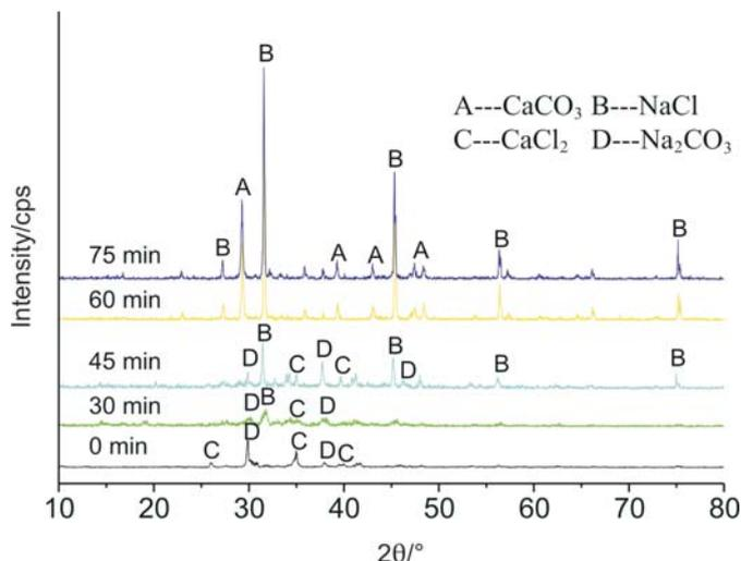
Figure 2 XRD spectra of the ground mixtures of CaCl<sub>2</sub> and Na<sub>2</sub>CO<sub>3</sub> at different times.
