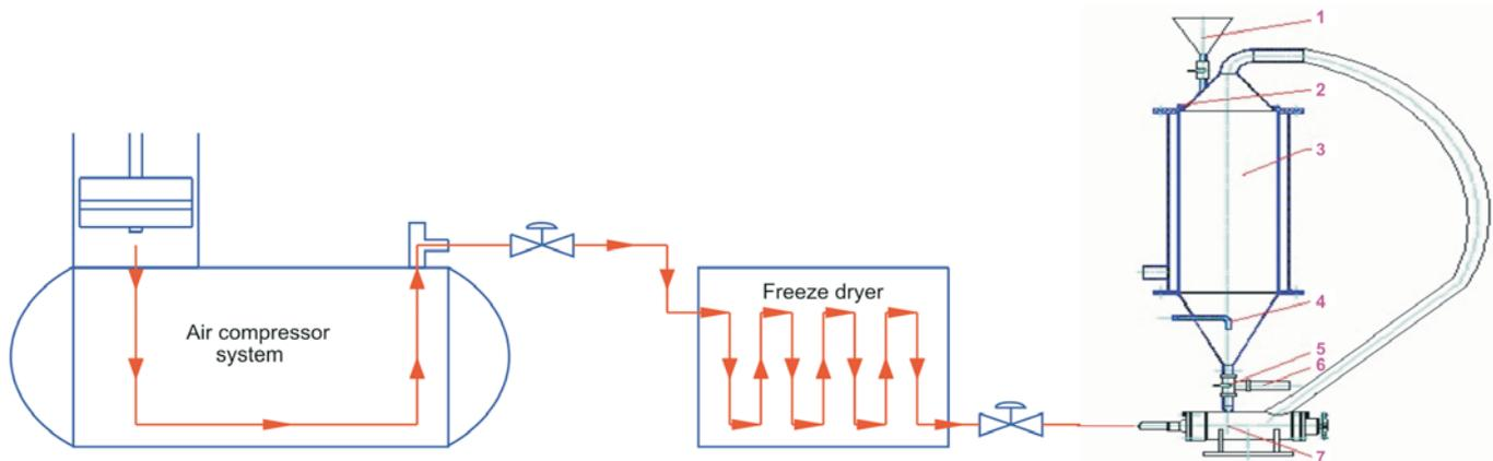
1, loading hopper; 2, delivery valve; 3, circulation collecting system; 4, adjustable jet pipeline; 5, tee globe valve; 6, outlet port; 7, reaction zone.
