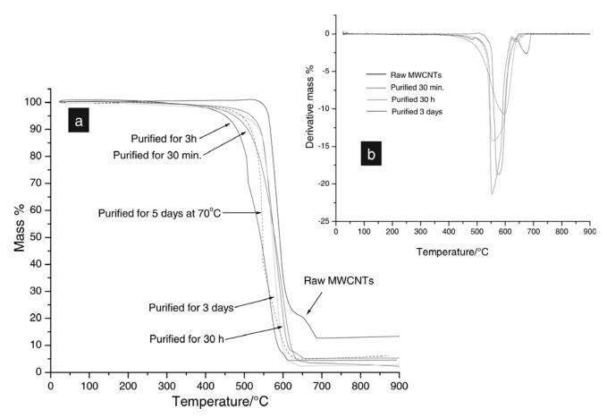
Figure 11 TGA profiles of (a) crude and purified CNTs synthesized from IMPN catalysts and (b) corresponding derivative profiles.
