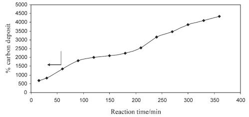
Figure 8 Graph showing the amounts of CNTs produced after different reaction times using IMPN catalysts (T = 700 °C).
