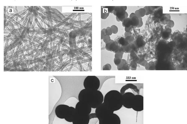
Figure 7 Low magnification TEM images of the carbon deposit produced with different dilution ratios of feedstock gases: (a)  $C_2H_2$ : $N_2 = 1:2.7$  (100 % CNTs), (b)  $C_2H_2$ : $N_2 = 1:1$  (CNTs and CMSs), (c) pure  $C_2H_2$  (CMSs and CNFs); T = 700 °C, t = 1 h.
