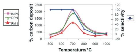
Figure 5 Graph showing the amount of CNTs produced and the percentage selectivity at different reaction temperatures in the CVD of C2H2 diluted with  $N_2$  ( $C_2H_2$ : $N_2 = 1:3$ , t = 1 h). The selectivity profile is similar for all the supported catalysts.
