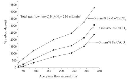
Figure 6 A graph showing percentage C obtained by varying the gas flow ratio of C<sub>2</sub>H<sub>2</sub> to N<sub>2</sub>. The synthesis time was 1 h for all reactions and the reaction temperature was 700 °C.
