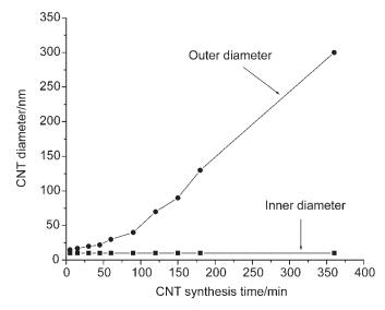
**Figure 10** A plot of variation of the CNT diameter with time for CNTs synthesized over IMP Fe-Co/CaCO<sub>3</sub> catalysts.
