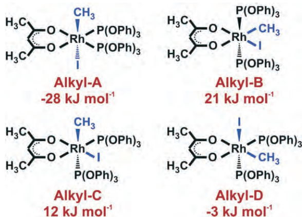
Figure 5 Four possible [Rh(acac)(P(OPh) _3 ) _2 (CH _3 )(I)] reaction products of the [Rh(acac)(P(OPh) _3 ) _2 ] + CH _3 I reaction with PW91/TZP/methanol calculated energies ( \Delta E_{TBE} ) listed below each alkyl. Alkyl-A (lowest energy) result from trans addition, alkyl-B, alkyl-C and alkyl-D represent the various cis isomers. Energies of reactants are taken as zero.
