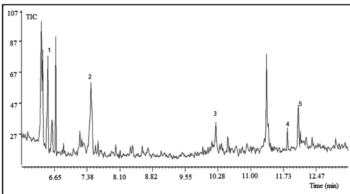
**Figure 8** A typical chromatogram of the Blaauwpan water sample extracted by SPE and detected by GC-MS. Where: 1 = Naphthalene, 2 = acenaphthene, 3 = phenanthrene, 4 = fluoranthene, 5 = pyrene.
