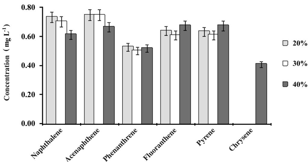
Figure 6 Effect of the amount of the conditioning solvent on the amount extracted.
