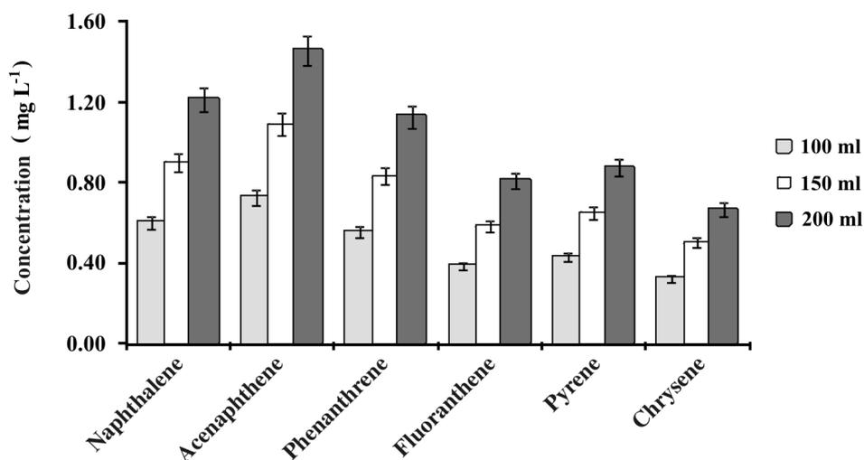
Figure 2 Effect of sample load volume on the amount extracted.
