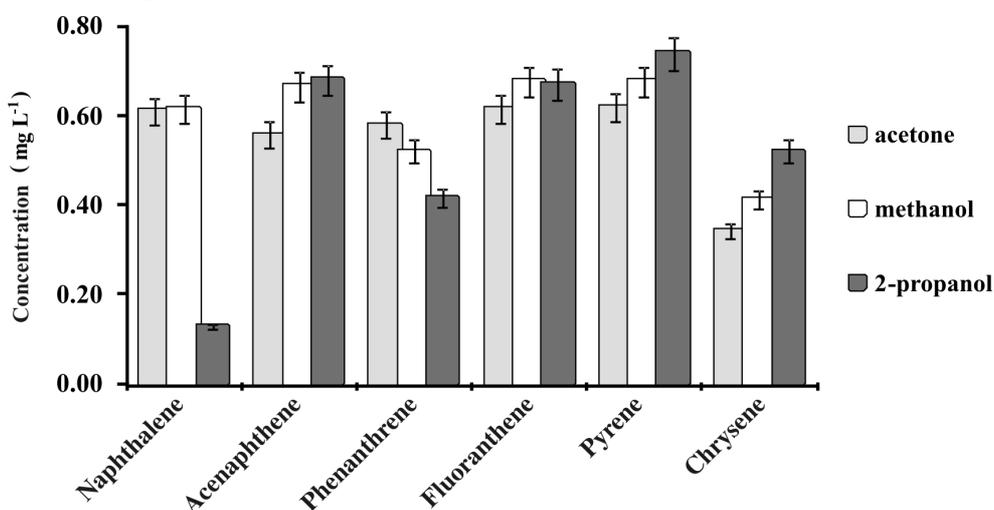
Figure 5 Effect of the conditioning solvent on the amount extracted.
