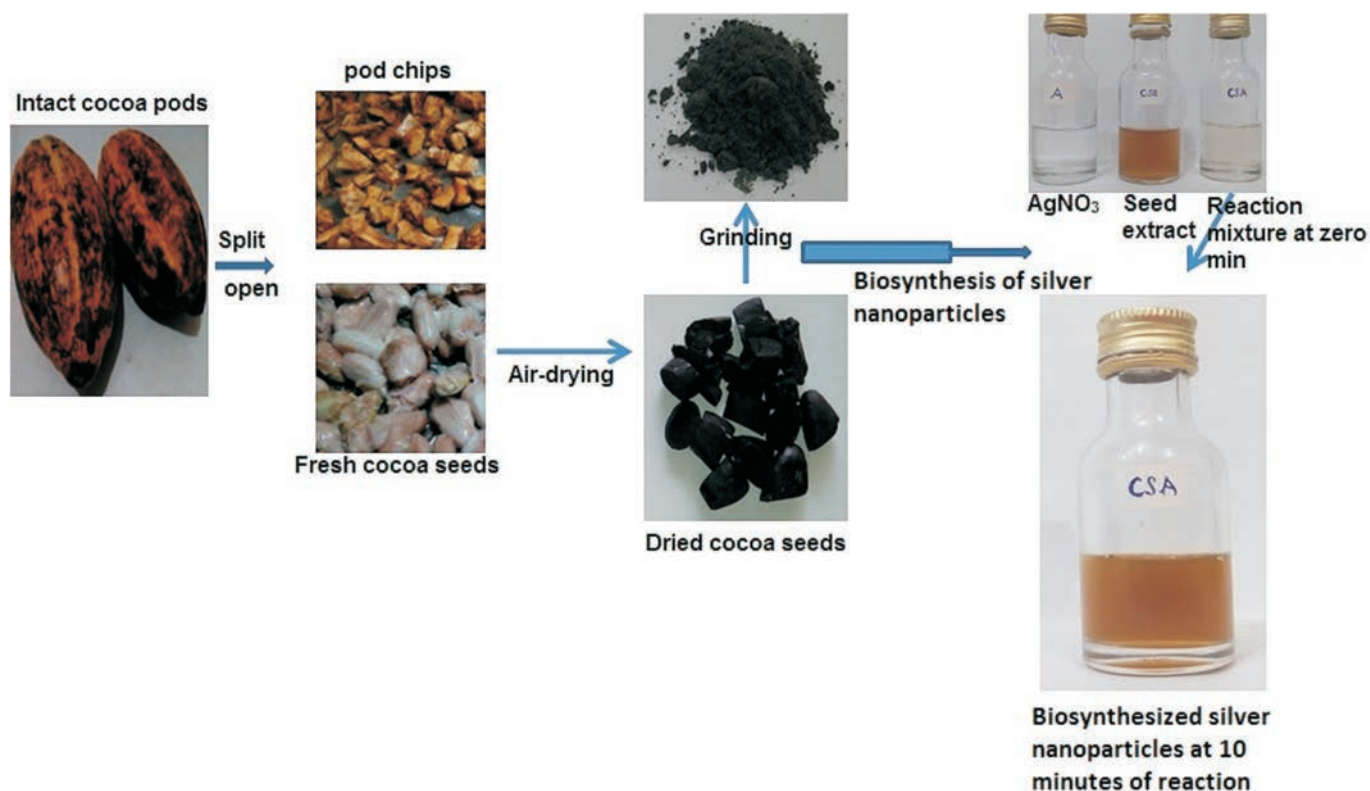
Figure 1 Scheme for the biogenic synthesis of AgNPs using the pod extract of cocoa.
