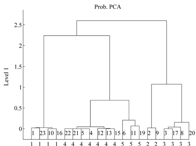
**Figure 6** Dendrogram of South African clinkers constructed from the two-dimensional latent variables. The *y*-axis shows the distances between clusters. Numbers at the bottom are the factory codes, while numbers within the dendrogram are the sample codes.
