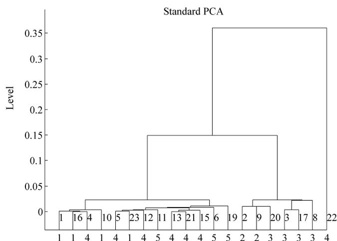
**Figure 4** Dendrogram of South African clinkers constructed from data projected into the first two principal components. The *y*-axis shows the distances between clusters. Numbers at the bottom are the factory codes, while numbers within the dendrogram are the sample codes.
