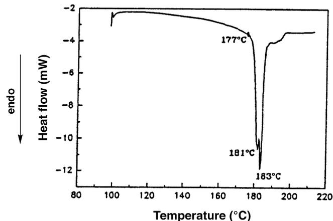
Figure 3 DSC trace for the 4 · DMSO enclathration complex (heating rate: 2.5 K min<sup>-1</sup>).
