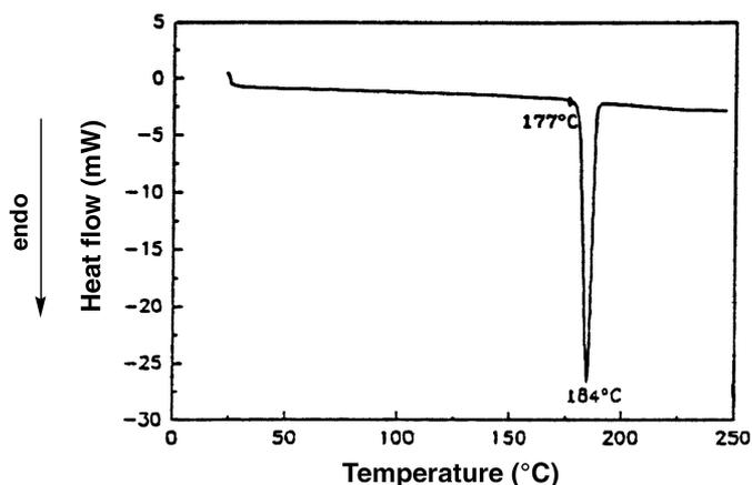
Figure 2 DSC trace for the 4 · DMSO enclathration complex (heating rate: 5 K min<sup>-1</sup>).
