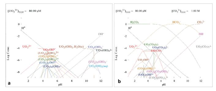
Figure 4 Speciation of uranium in a uranium-water system at 25 °C and I = 0 M (a), and in the presence of carbonates (b), calculated using Hydra and Medusa speciation modelling free ware versions.
