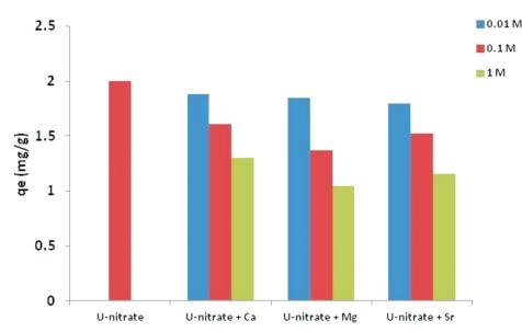
**Figure 5** Effect of  $Ca^{2+}$ ,  $Mg^{2+}$  and  $Sr^{2+}$  on the adsorption of uranium (VI) (U- nitrate system(n = 3 and RSD < 10 %).
