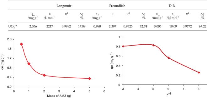
**Figure 2** Effect of AMZ mass on the adsorption of uranium (VI) (n = 3 and RSD < 10 %).
