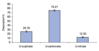
**Figure 6** Desorption percentage of U-nitrate, U- sulphate and U-carbonate adsorbed on AMZ (n = 3 and RSD < 10 %).
