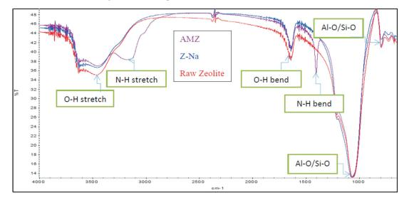
Figure 1 FTIR spectra of natural zeolite (raw zeolite - red), Z-Na (Na-zeolite - blue) and AMZ (purple).
