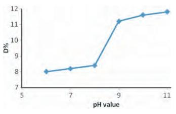
**Figure 9** pH-dependent adsorption of MB on powder surface, D(%)  $C_0$ ,  $C_e$ ,  $C_e$ ,  $C_e$ ,  $V_c \times 100$ , where D is distribution ratio,  $C_0$  means initial concentration of MB,  $C_e$  denotes equilibrium concentration.<sup>22</sup>
