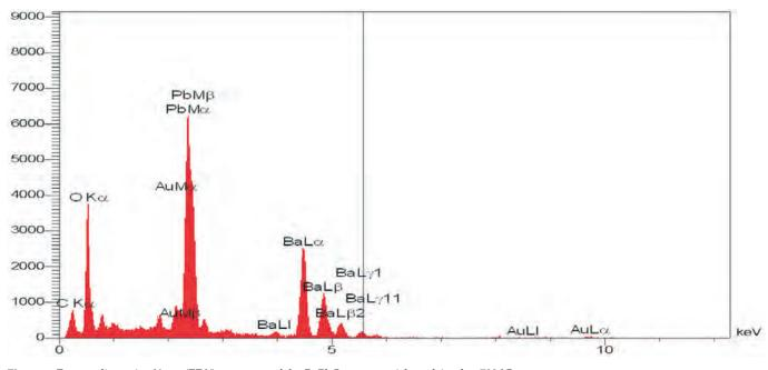
Figure 5 Energy dispersive X-ray (EDX) spectrum of the BaPbO<sub>3</sub> nanoparticles calcined at 700 °C.
