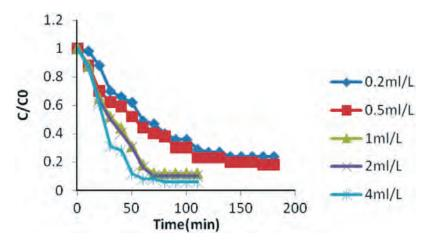
Figure 10 Decolorization of MB under different concentrations of H<sub>2</sub>O<sub>2</sub>.
