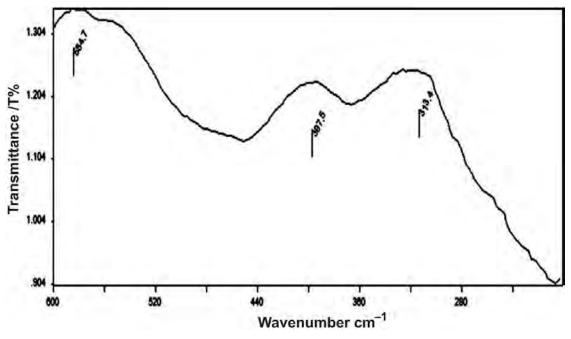
Figure 3 IR spectrum of BaPbO<sub>3</sub> calcinated at 700 °C.
