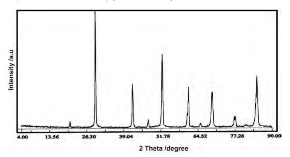
Figure 2 XRD pattern of BaPbO<sub>3</sub> nanoparticles calcined at 700 °C.
