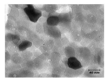
Figure 6 TEM image of BaPbO<sub>3</sub> calcined at 700 °C.
