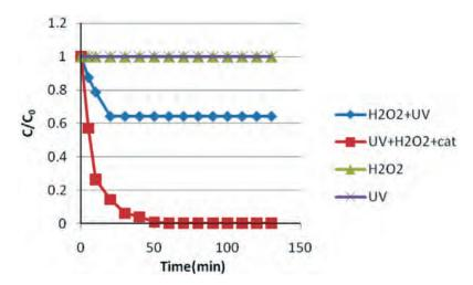
Figure 11 Decolorization of MB under 0.2 g 100 mL<sup>-1</sup> cat, 0.05 mL L<sup>-1</sup> H<sub>2</sub>O<sub>2</sub> and UV irradiation.
