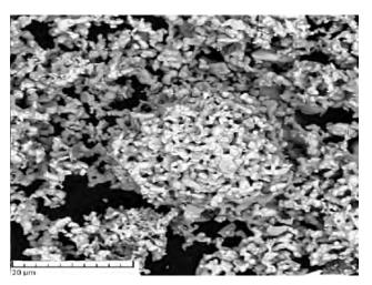
Figure 4 SEM image of BaPbO3 calcinated at 700 °C.
